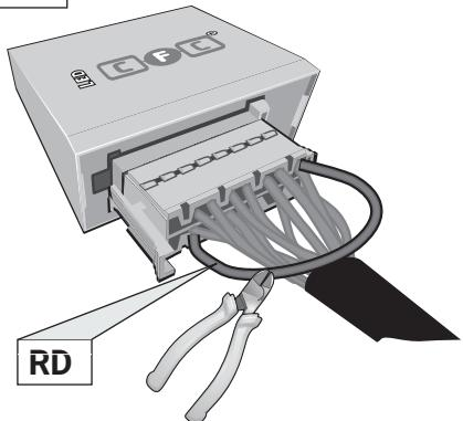
Pin 11 and Pin 2 disconnected
