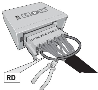
Pin 11 and Pin 2 disconnected
